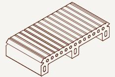
For this project, inaugurated for the XVIII Mediterranean Games, **Flexbrick®** created a new ad-hoc piece for the ventilated roofing. This allows for a noticeable improvement in its thermal insulation, with the corresponding energy savings, and it contributes to reducing the heat-related wear and tear on the weatherproof sheets.
