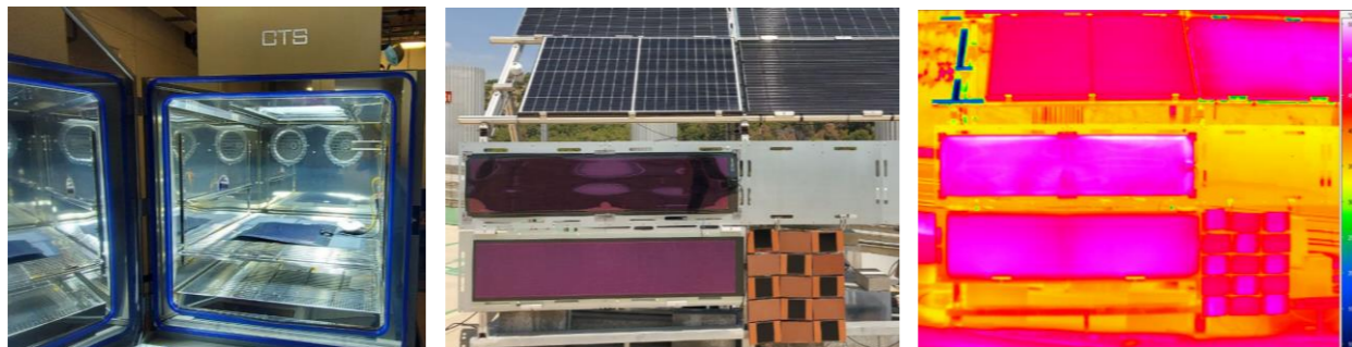
Indoor and outdoor tests of HeliaFilm modules, and image of their thermal Characterization.
