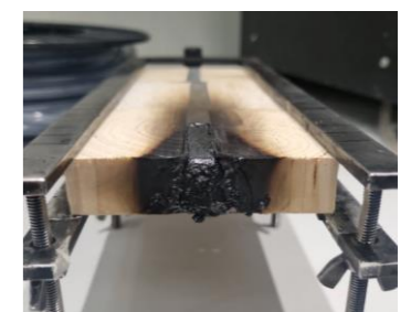
Small flame edge exposure for 30 s results in ignition of the flexible joint and dropping of flaming material.
