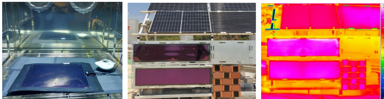
Indoor and outdoor tests of HeliaSol modules, and image of their thermal Characterization.
