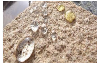
Hydrophobic Coating by TECNAN applied to porous building materials
