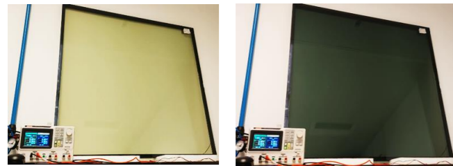
Dynamic variation of the visible transmittance of the Chromogenics ConverLight® 75 TGU under the application of three different bias voltages.
