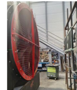
Set-up of the dynamic wind load test
