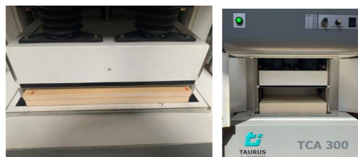
Sample measurement process with the Taurus TCA-300 device
