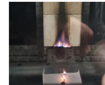
Small flame edge exposure for 30 s results in ignition of the flexible joint and dropping of flaming material.
