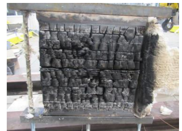
Flexible joint in tension after fire resistance test: unexposed side (left), exposed side (right).
