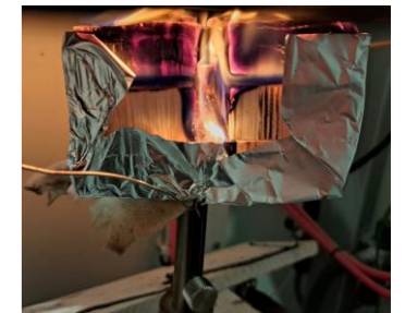
Cone calorimeter test of flexible joint – simulation of reduction of material.
