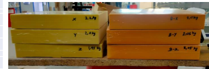
Probes X - Z / BX - BZ: High density PUR and bioPUR foam probes
