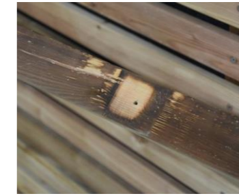
Minor discolorations and chipping after artificial ageing.
