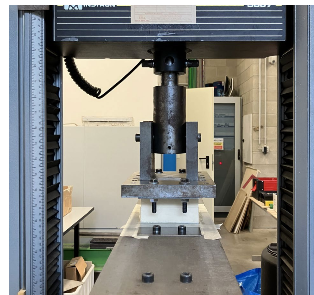
Cross panel tensile strength test setup
