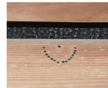
Minor dent and discoloration at the point of impact of the steel ball.
