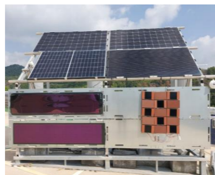
Indoor and outdoor tests of Flexbrick modules, measuring their characteristic IV and PV curves.
