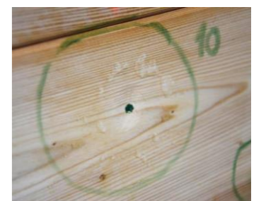
Minor dent and edge chipping at the point of impact of the ice ball.
