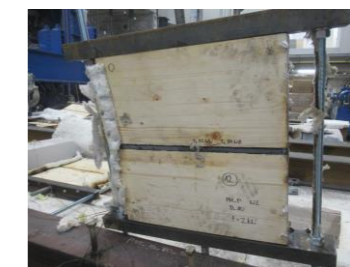
Flexible joint in tension after fire resistance test: unexposed side (left), exposed side (right).
